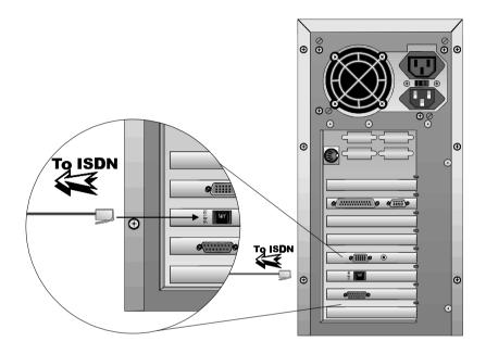
FIGURE 2-1: CONNECTING THE ISDN LINE
